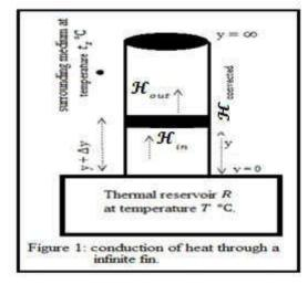
$t''(y) - \frac{\sigma^{\mathbb{P}}}{1P}[J(y) - t_s] = 0$  ...... (a), where Let us consider that the one end of the fin is connected to a heat source at y = 0 and the other end at  $y = \infty$  is free for losing heat into the surroundings. The source of heat is maintained at fixed temperature 'T' and t is
