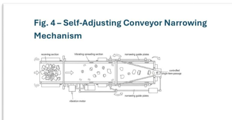
Figure 4. Self-Adjusting Conveyor Narrowing Mechanism for Waste Singulation (Addresses Gap 2)
