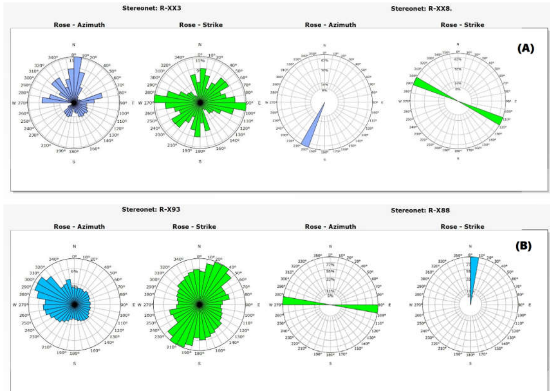
Figure 16: Dip and Azimuth for A- The wells under study, B- The other wells in the same pad
